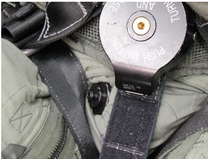
Anti-Exposure/Chem Bio Suit Adapter Shown integrated with flight suit for F-35 Harness
